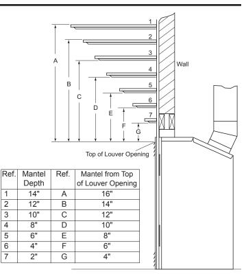
Figure 6 - Clearances for Combustible Mantels
